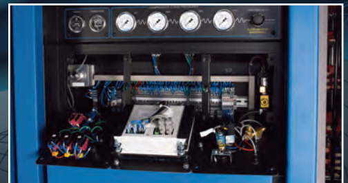
Hinged, "knockdown" sub-panels for routine maintenance and adjustments
